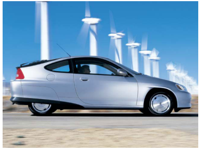
Fig. 8. Honda Insight with Kammback rear design [15]
