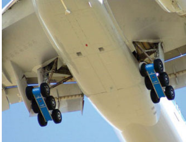
Fig. 4 Shielding on Landing Gear of Boeing 777 [12]
